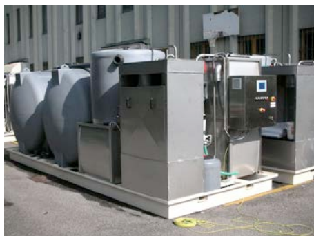
Figure 5: Mixed technology MBBR plants + MBR
