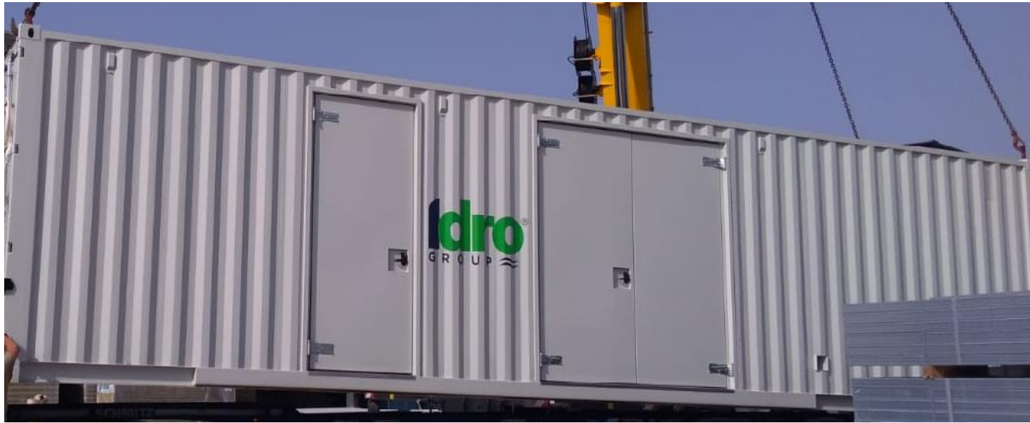
Filtration Unit - Oil Separator Plant in container for Rainy water with traced of oil and sand 25m3/h
