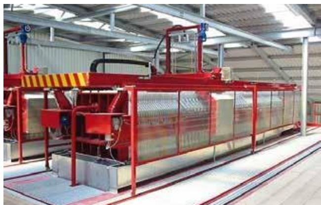
Filter press for sludge dehydration.
