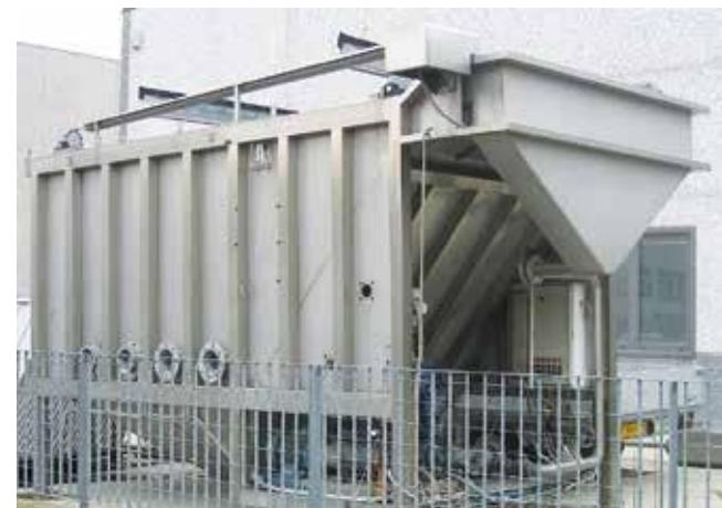
Flotation plant -  $Q = 1000 \text{ m}^3/\text{h}$ .
