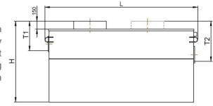
Apparatus NF certified by the CSTB (Scientific and Technical Centre for the Building industry), according XP P16 451-1/CN, CE marking (EN 858-1 standard). Opening with total accessibility, to facilitate the maintenance. (For extension shafts to contact our office. The article references below include step steady cover(s)). Ventilation DN75, for safety.
